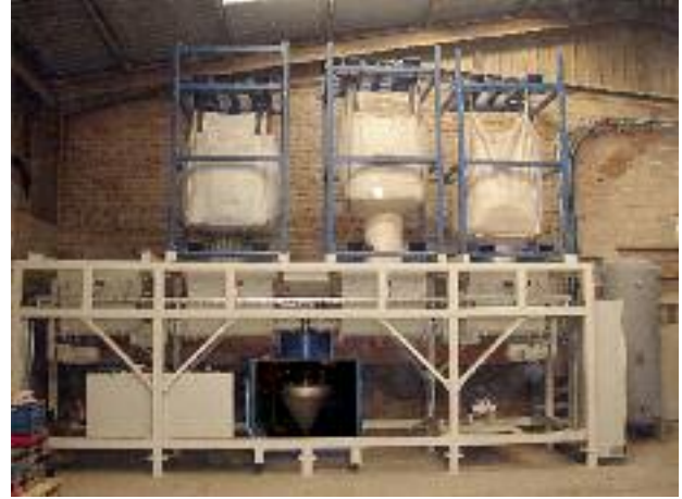
▲ FLEX 70 with one weighing/pressure vessel for low profile design and diverter valve in 2 mixers
