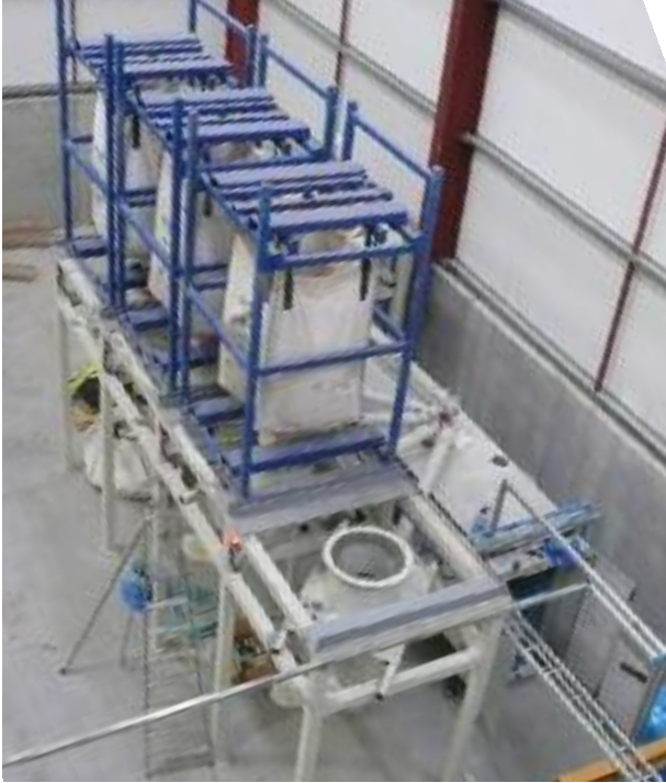
◀ FLEX 70-2 with 2 pressure vessels for 5 colors in 2 mixers
