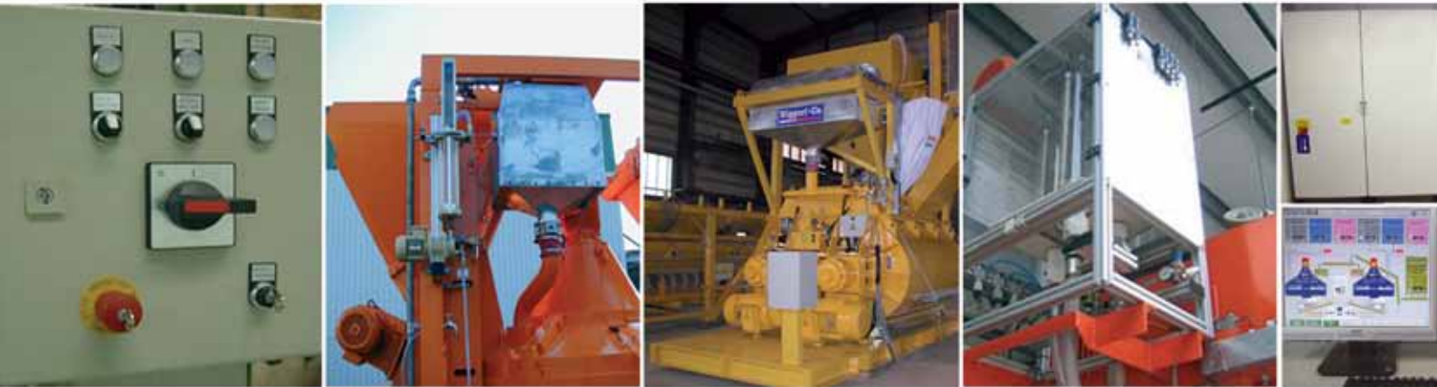
Mixer platform: Mixer with cement weigher and water weigher (as an alternative water addition via water counter); DWM – the alternative to the HPGM with ice weigher, admixture weigher
