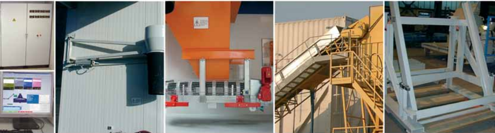
Concrete discharge: swivelling chute for concrete discharge into truck, extraction belt for concrete
