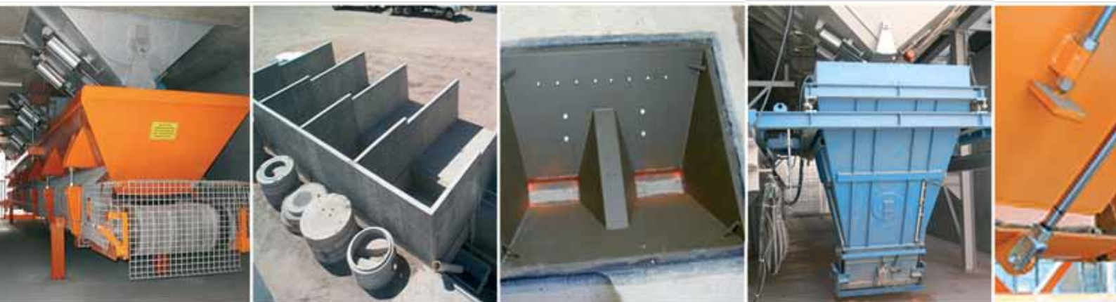
Aggregate weighing: optional aggregate silo made out of concrete with weigh-belt suspended from the ceiling and dosing cones for coarse/fine dosing, Movable weigher – the alternative to the weigh-belt
