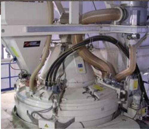
McGuire chose a combination of ACT systems for the new facility, including the Wiggert MobilMat MO80 - 5 - PCS with a high intensity planetary countercurrent mixer, and a fully automatic Würschum COM 70-3 pigment metering system.
