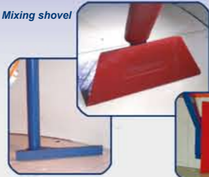
Mixer cleanout aid for faster discharge and shorter cycle time.
