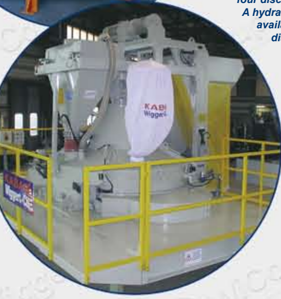
Module unit with skip hoist and cement weigher
