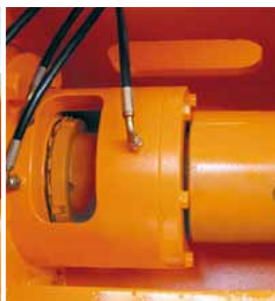
Automatic central lubrication system
