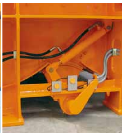
Oversized discharge gate with two hydraulic cylinders
