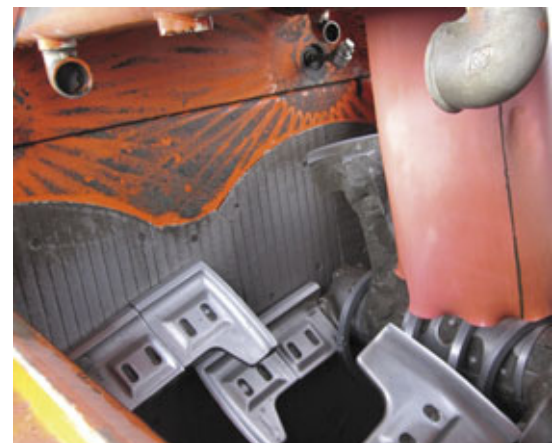
The power of automated high pressure washout system – after 3 weeks of use without manual cleaning, this Wiggert DWM 4500 twin shaft mixer, the heart of VanHooseCo’s central mix batching plant, is fitted with an automatic mixer cleaning system.
